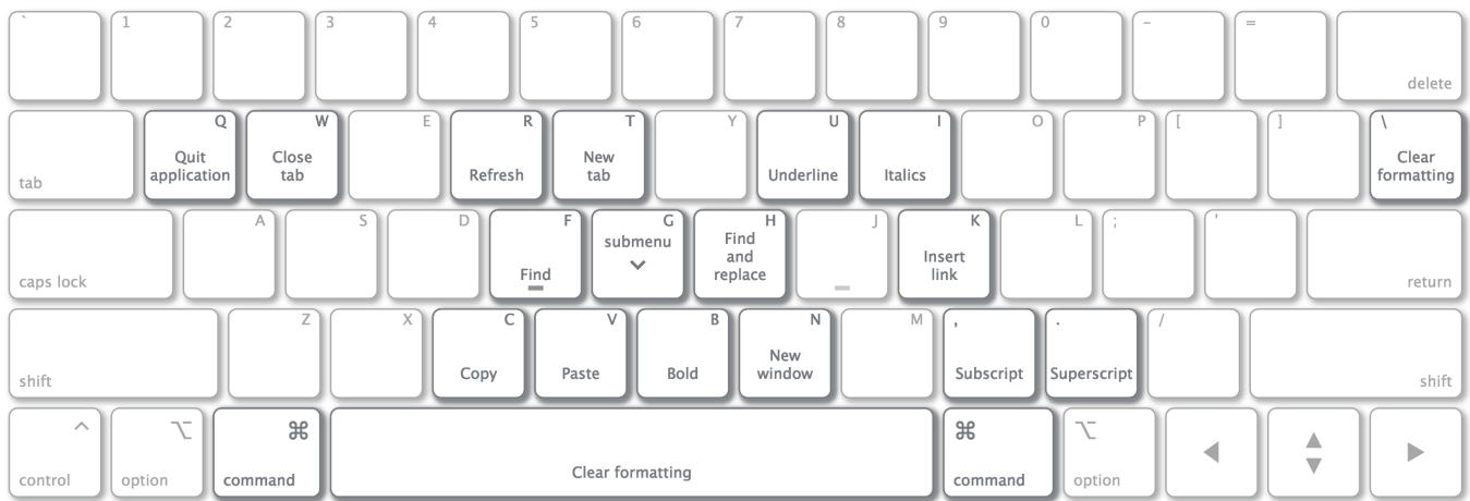
Figure 2. Example KeyMap interface shown while the Command modifier is held down, each shortcut key associated with Command is rendered with the name of the corresponding application command.
